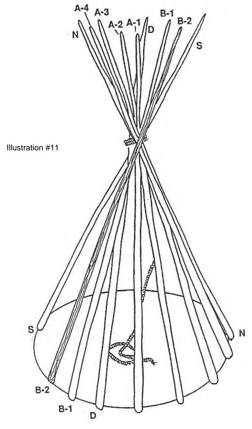
15. B-3 and B-4 go one on top of the other poles in the same crotch. Proceeding around the circle toward the S pole, set the base of B-3 and lean it in on top of B-2; then B-4 on top of B-3, keeping the bases of Group B evenly spaced between the D pole and the S poles.
