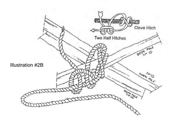
HINT—especially for large tipis—to prevent your tripod knot from slipping: After measuring for your tripod (Chart B) drill a  $\frac{1}{4}$ " hole (no larger!) through all three tripod poles and lace through it with a 5' piece of  $\frac{1}{4}$ " liner rope. Wrap it around the tripod a few times and tie it off.
