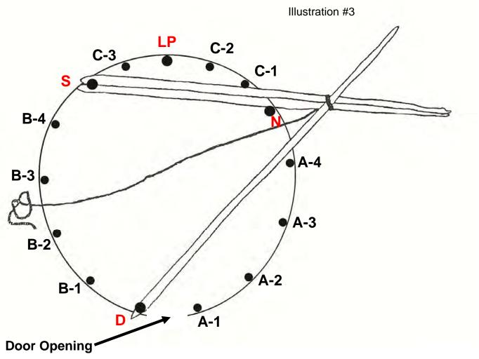
7. To raise the tripod, one person should place his feet against the bases of the N and S poles to keep them from "kicking out". A second person lifts the N and S poles together starting at the tips and walks them up. When the tripod is almost vertical, swing the N pole across to its proper spot (Illustration #4) and let the tripod rest on all three poles.
