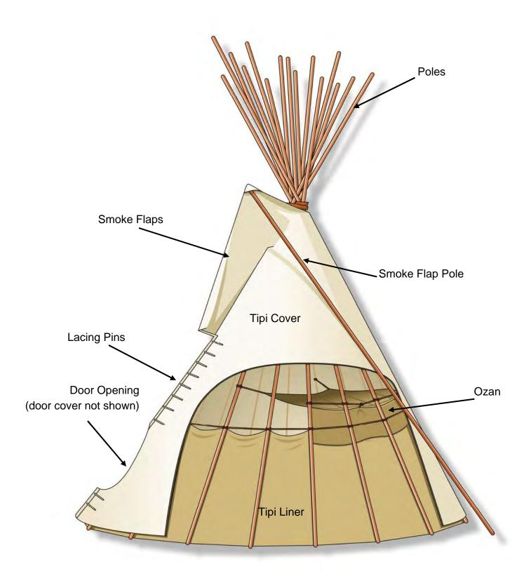
Tipi Components Cutaway View
