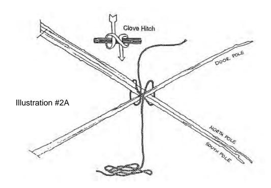
5. Use the tripod rope. Tie a clove hitch around all three poles. See Illustration #2A and #2B. Lock the clove hitch by tying two half hitches with the short end of the rope around the long end. Tighten the two half hitches against the clove hitch. MAKE SURE THE KNOT IS TIGHT SO IT WON'T SLIP. Don't cut off the leftover tripod rope after tying the knot; you'll use it later.
