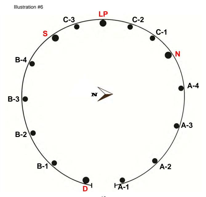
10. The four poles in Group A are placed with the base ends spaced between the D and N poles. Place A-1 a few feet north of the D pole and lean it into the cluster of poles at the top, specifically in the crotch formed by the N and S poles, which stick out over the front.
