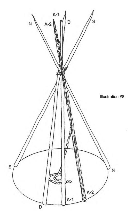
12. Poles A-3 and A-4 follow the same order, all in the same crotch, one on top of the other. Set the bases of the A group of poles so they are evenly spaced between the D pole and the N pole.
