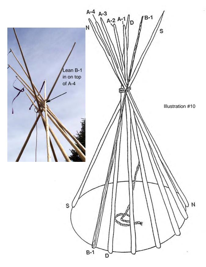
14. Place the base end of B-2 a few feet around the circle from B-1 and lean it into the cluster on top of B-1.
