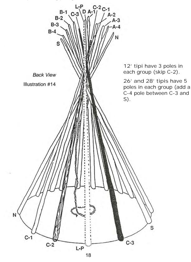
Now all the interior tipi poles—except the Lifting pole—are in place. You're ready to wrap the dangling tripod rope around them.
